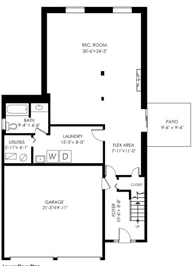
**Lower Floor Plan** Floor Area: 1081 sq.ft. Ceiling Height: 8'
