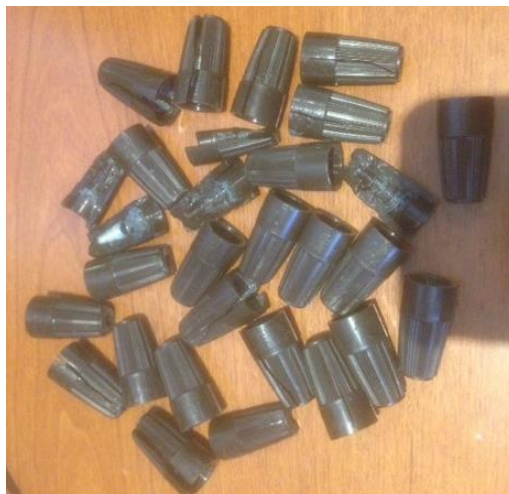
Figure F2 – Non-Petroleum based inhibitor failures
