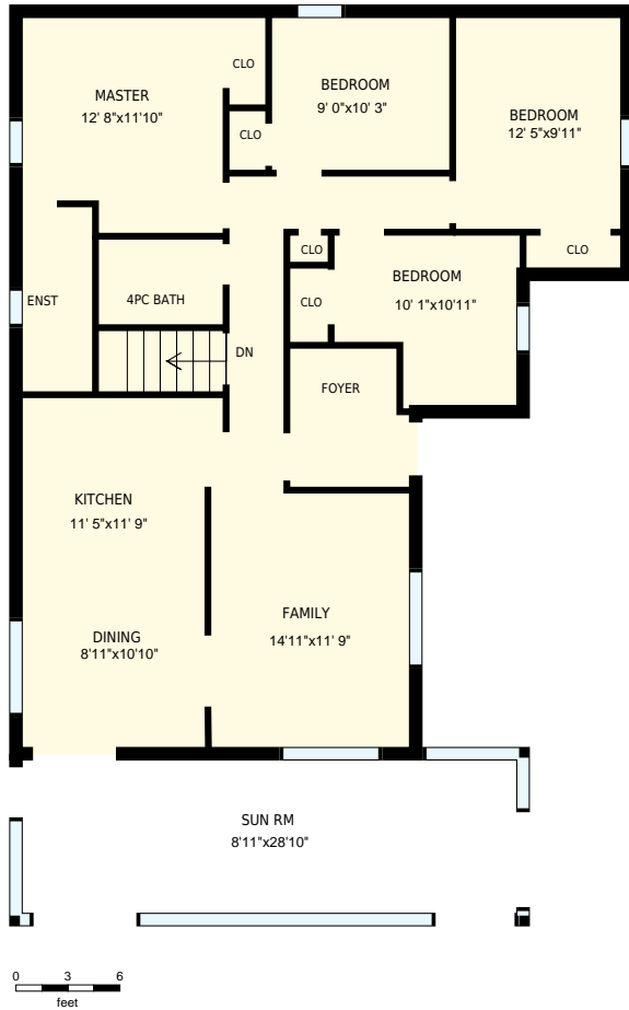
Main floor Exterior Area 1281 sq. ft.
