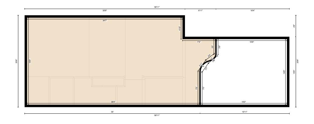
Measurement Diagram for: 2nd Floor Exterior Wall Thickness: 6.3 in
