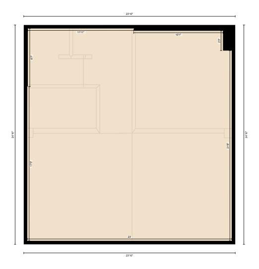
Measurement Diagram for: 1st Floor Exterior Wall Thickness: 4.5 in
