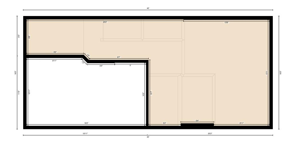
Measurement Diagram for: Main Floor Exterior Wall Thickness: 6.5 in
